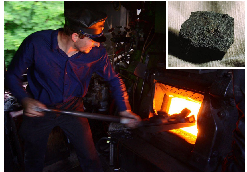
Fireman shovels coal into the engine of a steam-powered train. Image is courtesy of wikimedia commons and is public domain
