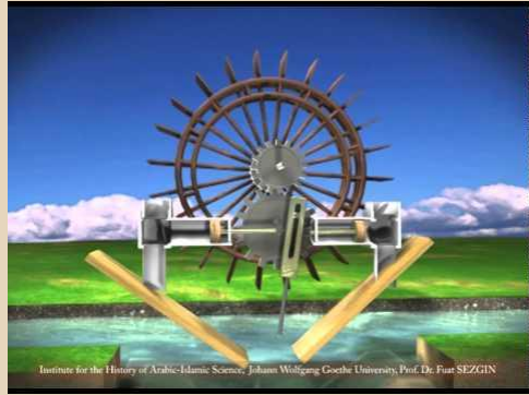
Water Wheel Pump
